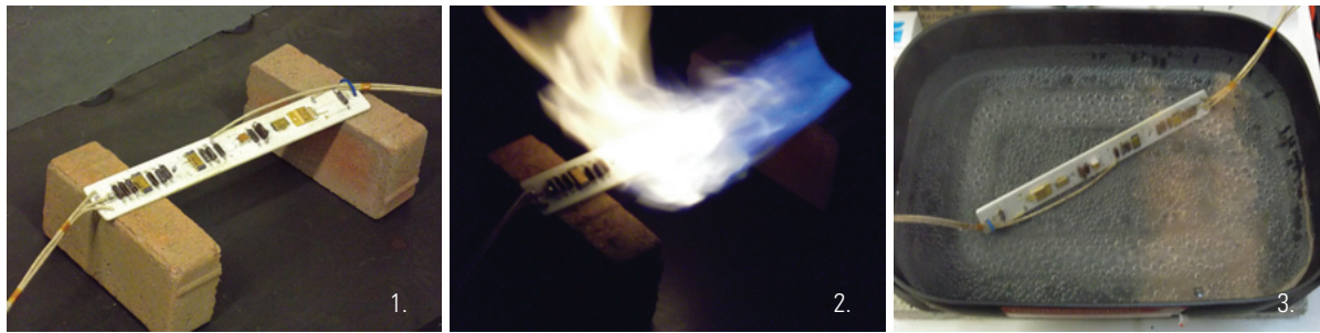
Figure 1. An actual working circuit, which can measure pressure or temperature in a geothermal tool. This circuit survived a thermal shock over 427° C (800° F) and boiled in brine.
