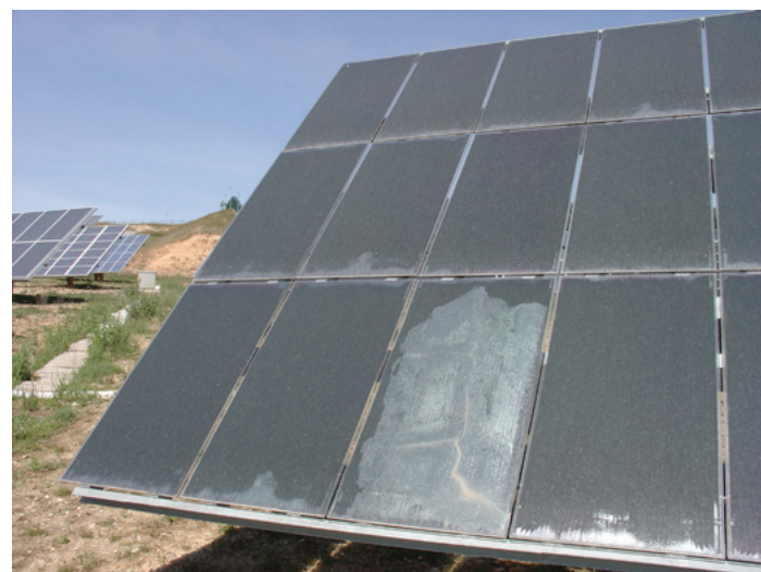
TCO corrosion in a superstrate amorphous silicon module.
